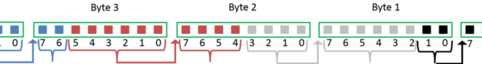
Figure 1. Packing two 10-bit pixels into three bytes.
