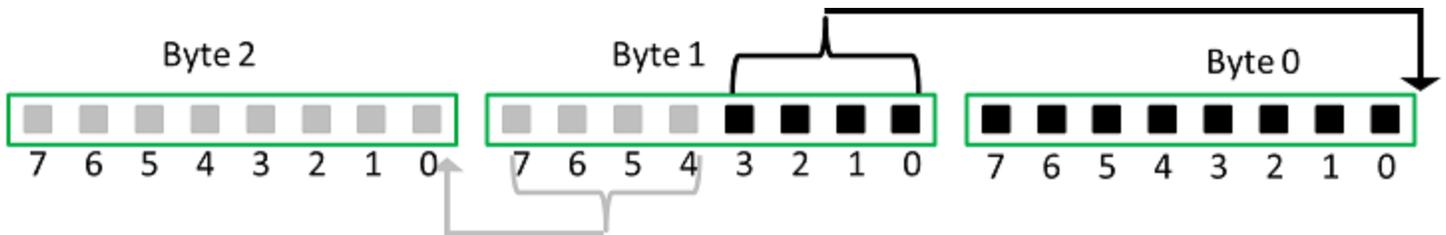
**Figure 4.** Packing two 12-bit pixels into three bytes.
