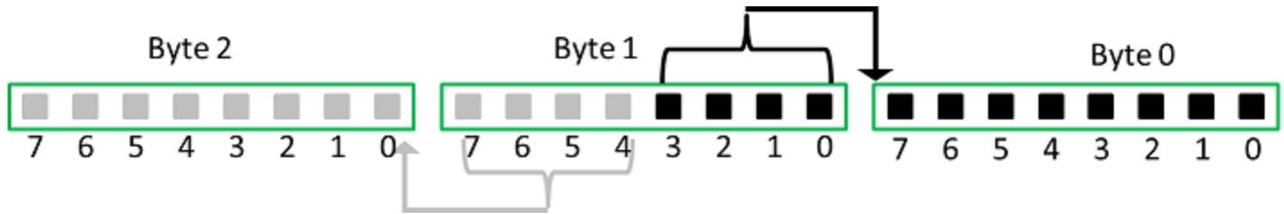
**Figure 3.** Packing two 12-bit pixels into three bytes.
