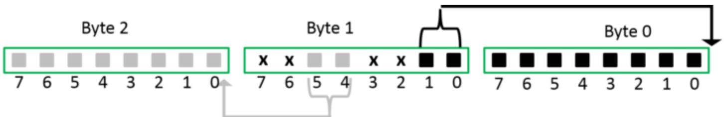
Figure 2. Packing two 10-bit pixels into three bytes.
