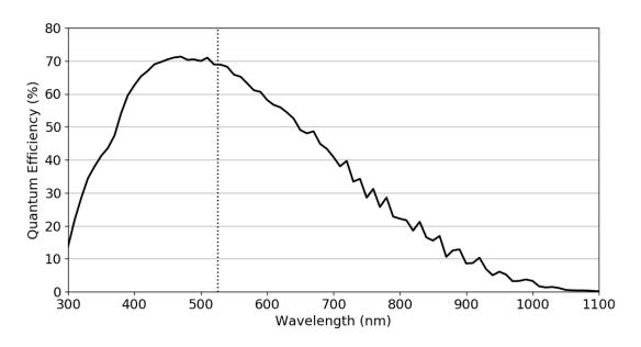
Forge FG-P5G-51S4C Spectral Response Curve
