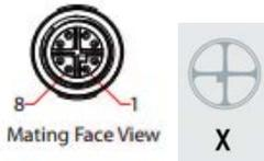
Plug the M12 X- coded USB3 cable into the camera and screw until tight. Securing the cable ensures a reliable connection and helps to keep moisture out of the camera.
